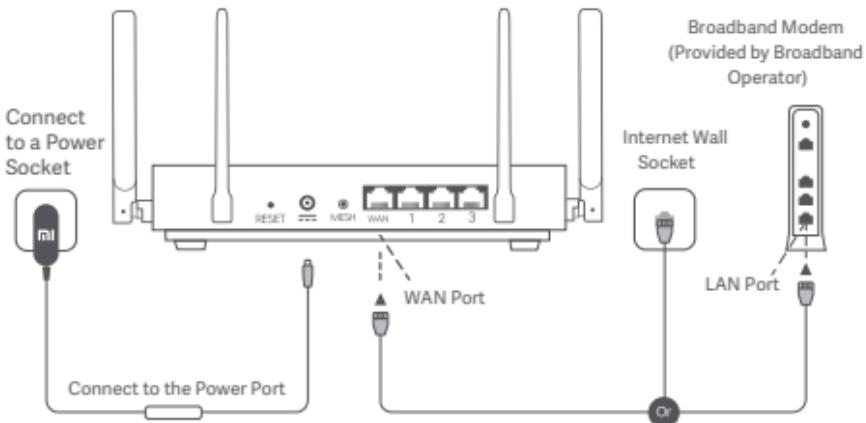
\*Broadband modem is provided by the broadband operator. If it is not available, you can connect the network cable to the router and the Internet wall socket, or directly connect the indoor network cable to the router's WAN port.
