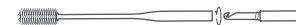
Cleaning Brush (Rotate the handle of the cleaning brush to remove the blade)
